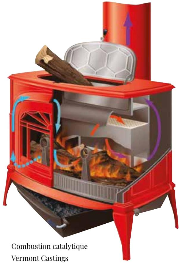
Combustion catalytique Vermont Castings
